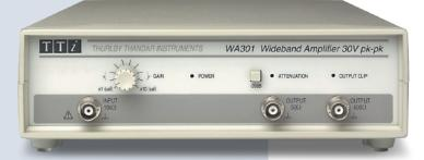
The WA301 wide-band waveform amplifier is intended for extending the maximum output voltage swing of function and arbitrary generators for applications where an EMF of 20 volts pk-pk is insufficient.
