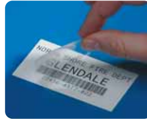
3. Laminate is applied over standard label.
