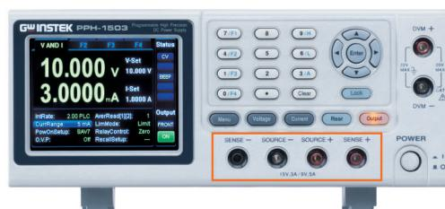
**Front Panel of PPH-1503 (Output Terminal)**
